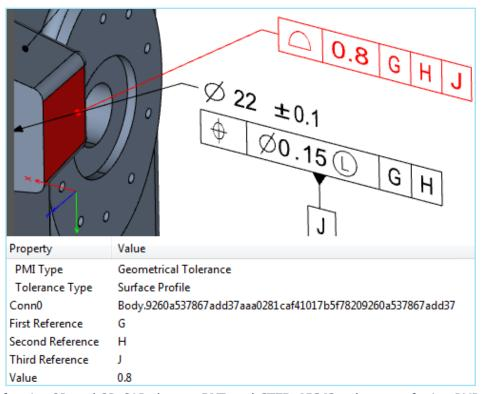
CrossManager is also supporting conversion of native 2D and 3D CAD data to **DXF** and **STEP AP242**... thus transferring PMI representation to standard CAD formats.
